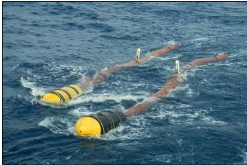
Fig: Deployment of Gun array for Seismic
