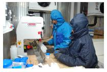
At NCPOR, the scientific endeavors are multidisciplinary in scope and content. The institute boasts of the country's only ice-core archival, processing and analytical facilities comprising an ultracold room at a temperature of  $-20^{\circ}$  C and a class 100 clean room.
